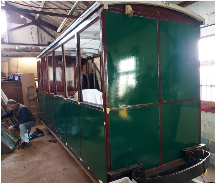
Preparing and filling exterior woodwork
